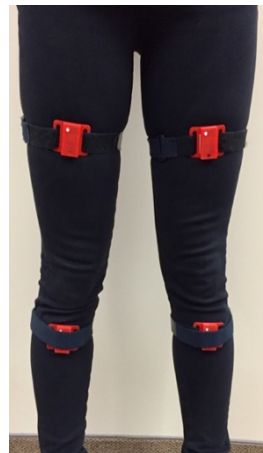
Figure 1: Example of wearable sensor positioning
