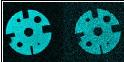
Figure 1. Original fully-sampled 1 H resolution phantom image (right, SNR=6.5) and nine averages image (left, SNR=22).
