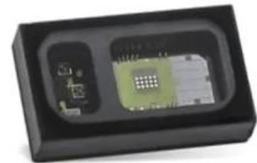
Figure 1: MAXM86161 PPG Sensor
